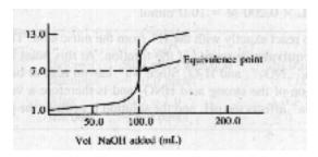
Notice the sharp slope around the equivalence point region - this is indicative of strong acid + strong base titrations. Note that the equivalence point pH is 7.0 - this is also what we would expect for this type of titration. Knowing how to predict the type of titration from a graph can be of considerable assistance to you in CH 223.
