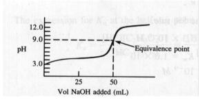
Note that the equivalence point is basic in a weak acid + strong base titration, a result of the conjugate base of the weak acid. Also note how the slope around the equivalence point is not as steep as it was when strong acids and bases were mixed together.
