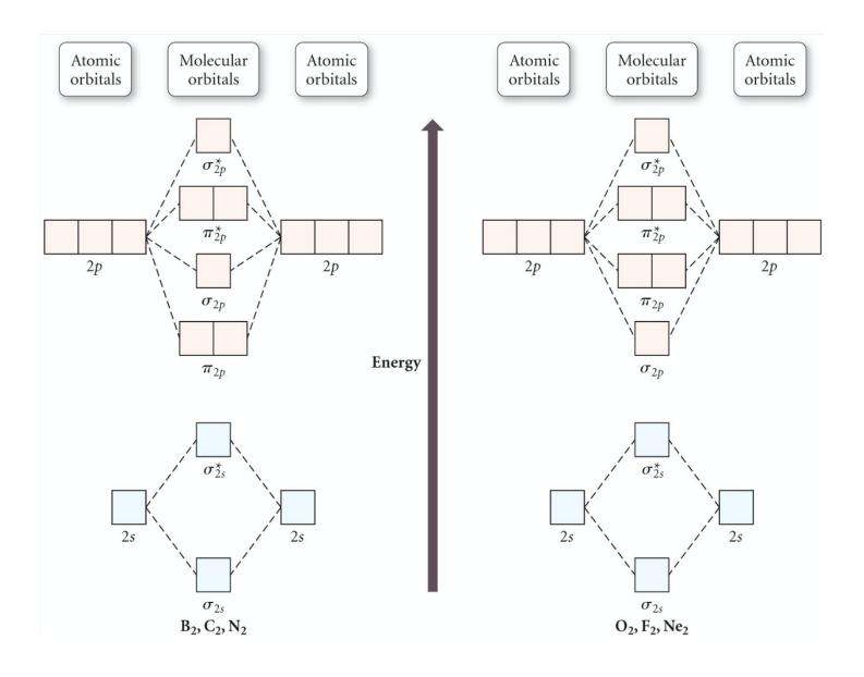
Molecular orbital diagrams for B, C, N (left) and O, F and Ne (right).
