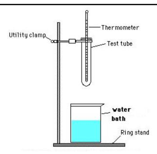
This picture should also include a hot plate under the beaker and a "swizzle stick" around the thermometer
