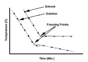
In both the pure liquid and the solution, a **supercooling** effect may be seen. As the solid begins to form, the temperature may drop *below* the actual freezing point initially and then come back up to the freezing point temperature as the solid forms. Supercooling is usually not observed if adequate churning of the sample is provided. When determining the freezing point, the super-cooling effect should be ignored.
